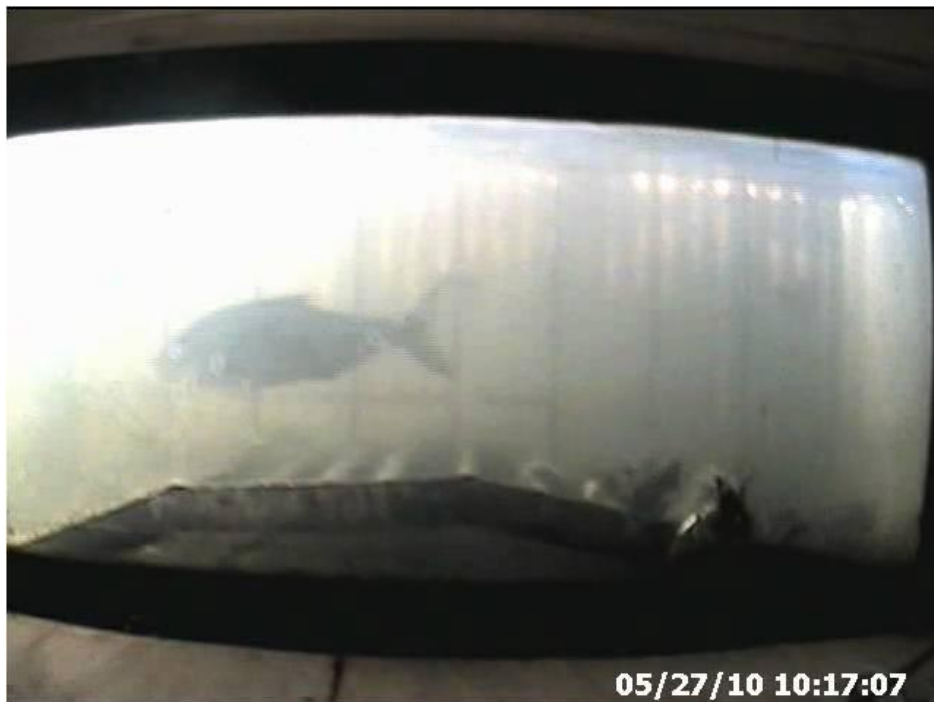
A photo snipped from the digital file at Kinneytown, showing a gizzard shad passing the window. The arched grating seen under the fish is designed to keep fish from passing under the lower lip of the window and avoiding detection by the camera.
